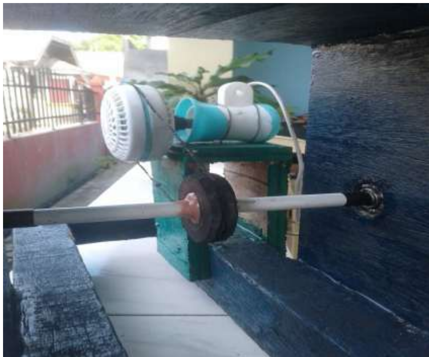
Figure 1.10 Belt, Pulley and motor
